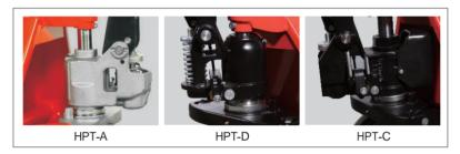
W Excellent design of hydraulic pumps, robust and durable, with fine contro( of lowering speed and overload valve, low routine maintenance.
